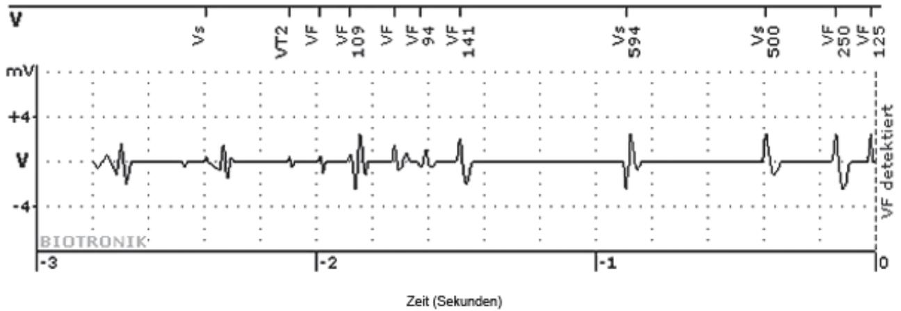
**Figure 1.** Signs of lead failure in remote follow-up technology. y-axis – amplitude in mV; x-axis – time before detection of arrhythmia in s. V – marker channel; Vs – ventricular sensing; VT2 – arrhythmia in the VT2 zone; VF – ventricular fibrillation; numbers (e.g. 109) time in ms.
