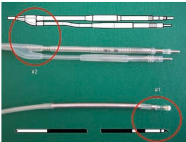
**Figure 4.** Schematic image and photography of an SF 6931 single coil electrode – vulnerable spots. #1 marks the tip conductor; #2 marks the pace sense ring conductor.
