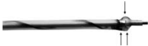
**Figure 1.** Thermography catheter with the thermistor on one side at the distal part (two arrows), and the hydrophobic construction at the opposite side (one arrow).
